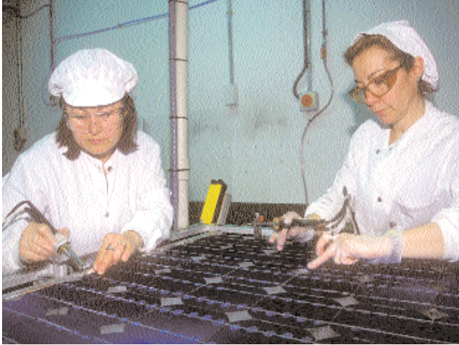
Soldering on: PV module matrix is soldered at a BP Solar plant BP SOLAR
